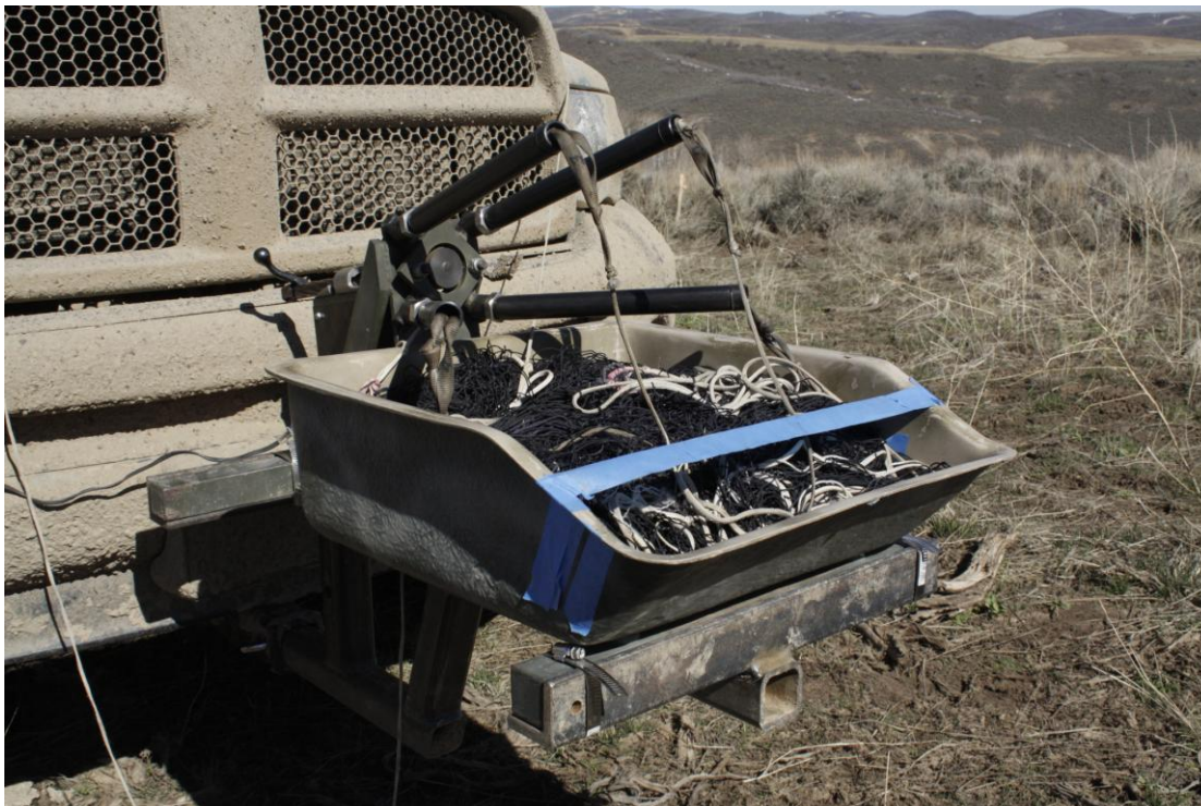
Figure 2. Bumper-mounted CODA net launcher used to capture greater sage-grouse.
